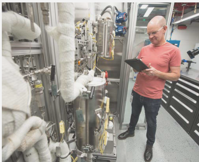
The FSCL lab manager adjusts operating conditions on a fixed-bed reactor system from his mobile device. Photo by Dennis Schroeder, NREL 51047
